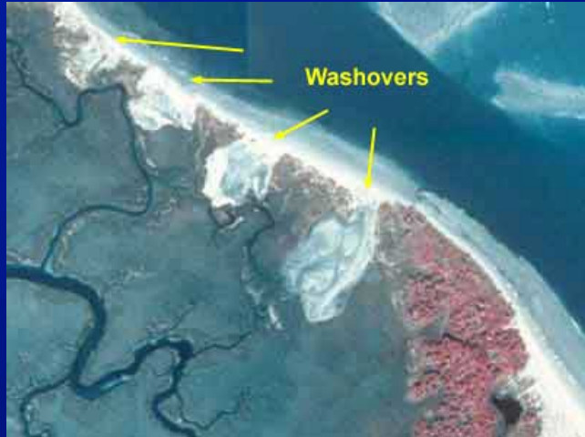
FTDs begin as storm overwash fans, which cut a path thru island
