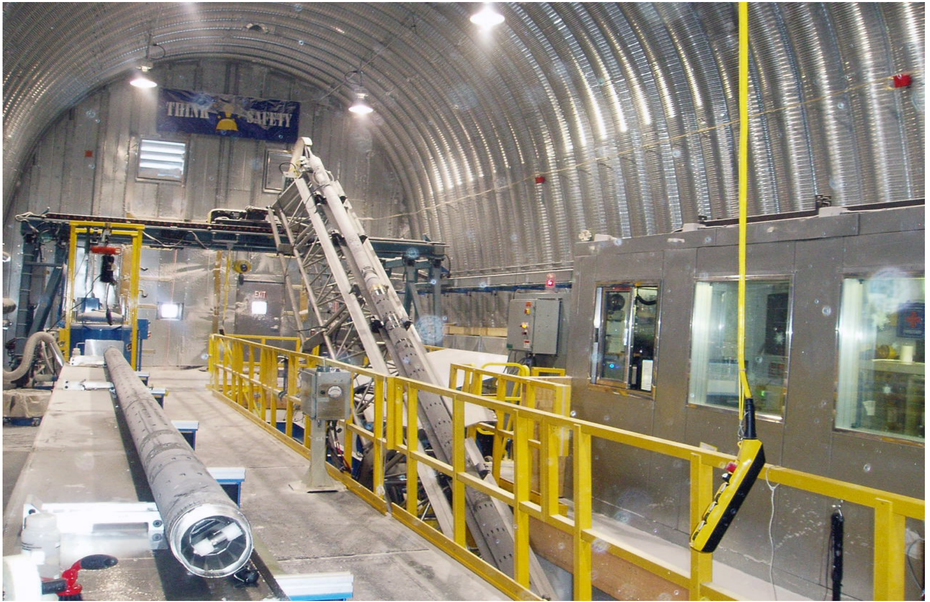
The DISC Drill's sonde and tower tilt from vertical to horizontal to aid in the removal of the ice core and chips. In this image the tower and sonde are at a \sim 45^\circ position inside the drill slot.
